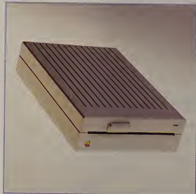
In comparison, the Apple drive is available in only one format—a single 5¼-inch 360K drive.
